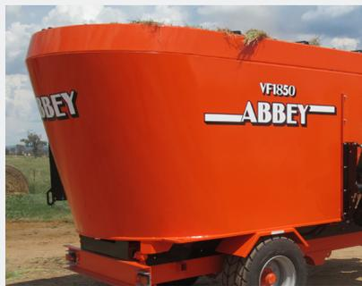
Rolled walls for superior mixing
