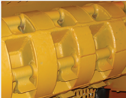
360 degree swinging hammer flails
