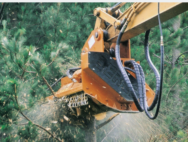
360 degree swinging hammer flails
