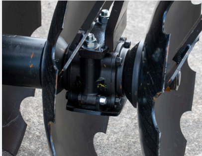
Double taper roller bearings with dual greasing and protectors
