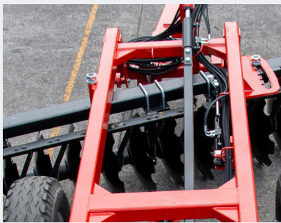
Hydraulic angle adjustment on front gang
