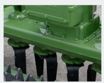
Fully welded gearbed
