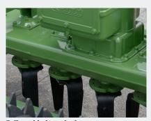
Fully welded gearbed
