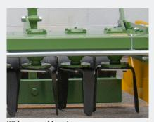
Wide spaced bearings on rotors
