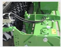
Leveling bar attached to gearbed
