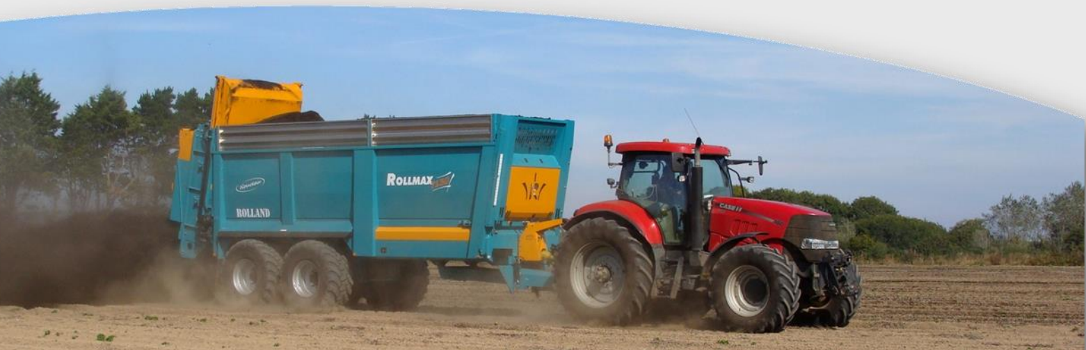
Drawbar with hydraulic suspension with accumulators for shock absorbers
