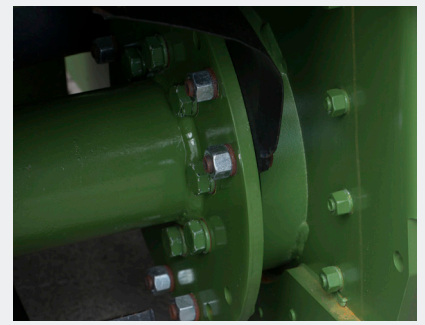
Steel face to face rotor seals
