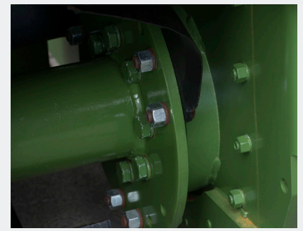
Steel face to face rotor seals
