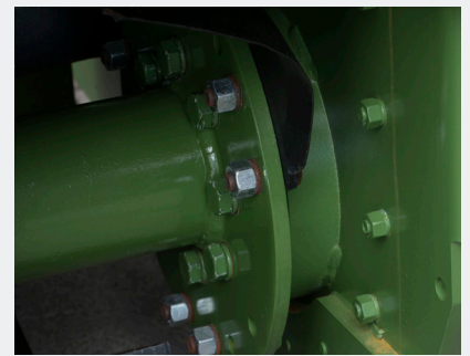
Steel face to face rotor seals
