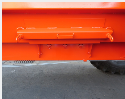
Watertight access hatch / stone trap
