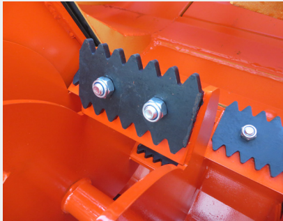
Replaceable teeth on rotor
