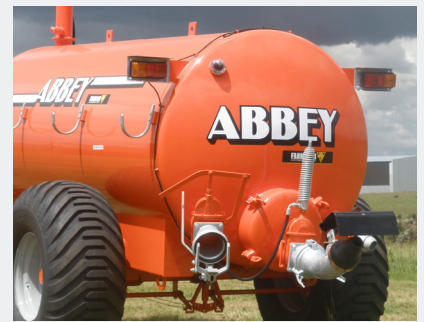
Pressed dome ends
