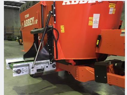
PVC elevator, low maintenance
