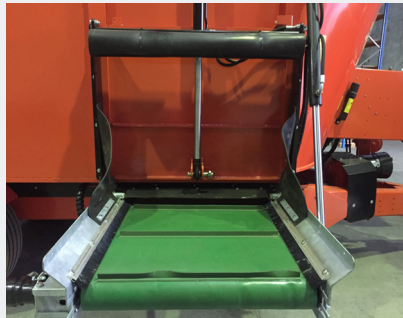
1m wide feed door for even feeding
